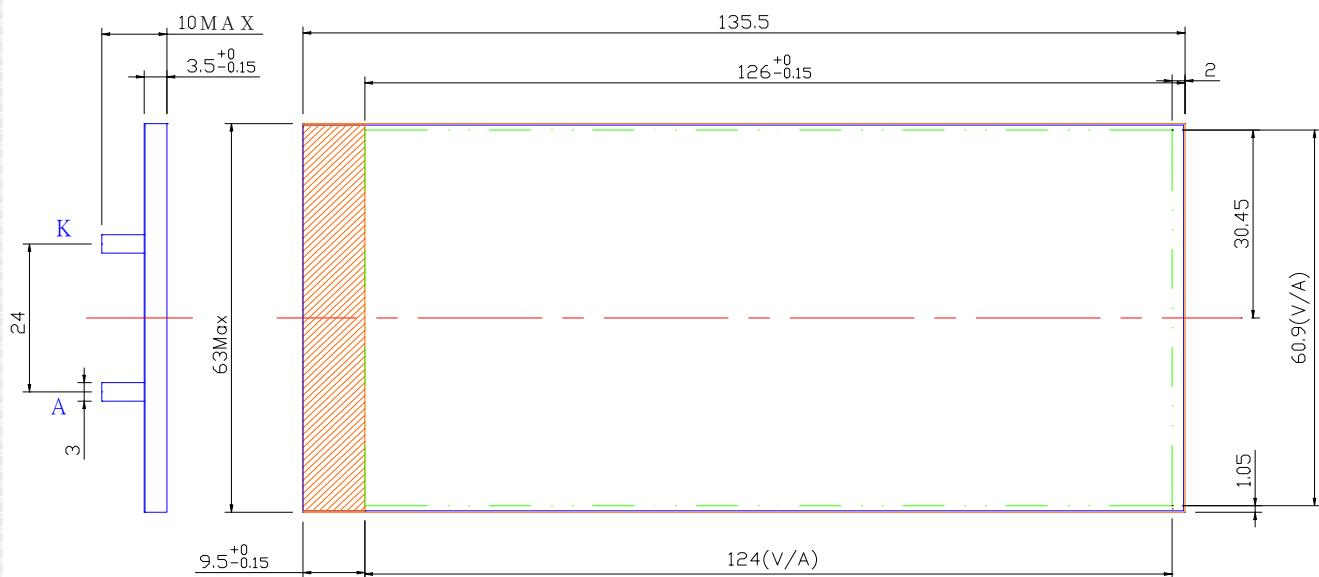
Note: Dimension in millimeters, and tolerance is  $\pm 0.35$  unless otherwise noted.
