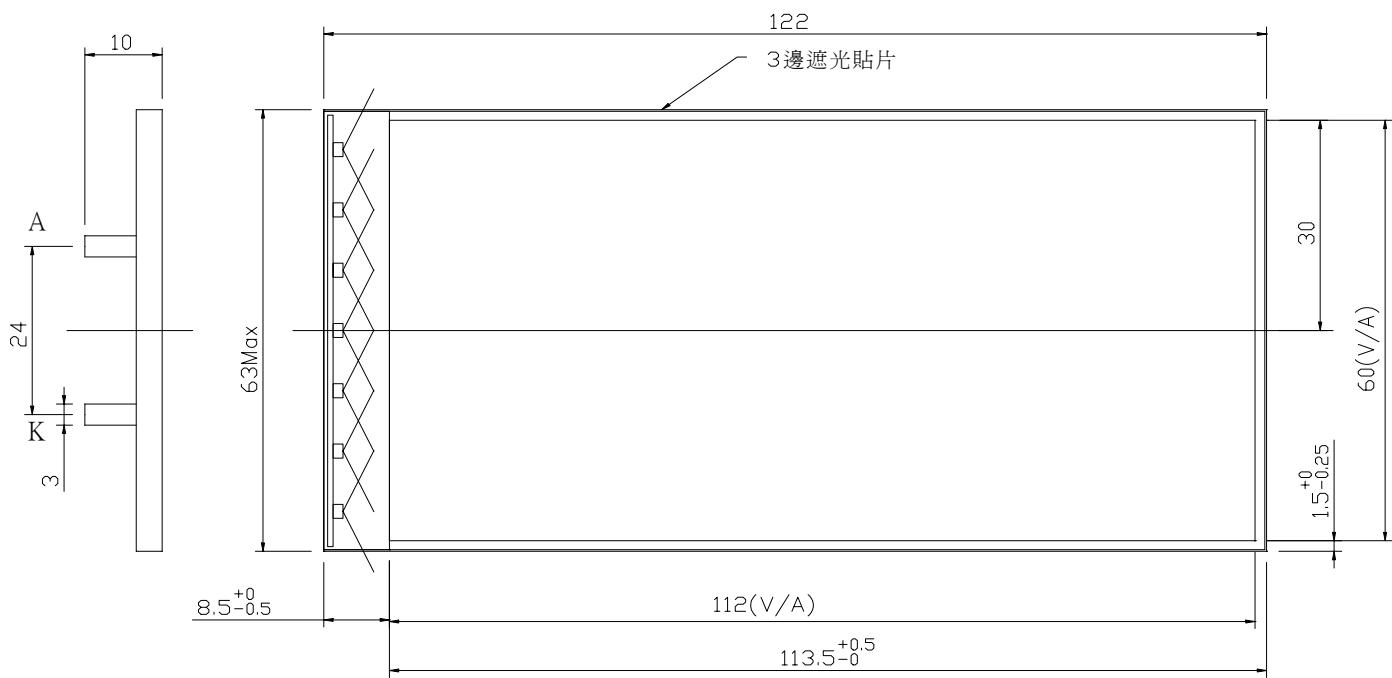
Note: Dimension in millimeters, and tolerance is  $\pm 0.35$  unless otherwise noted.
