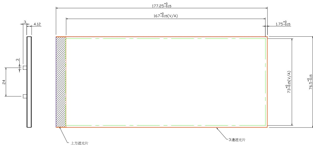
Note: Dimension in millimeters, and tolerance is  $\pm 0.35$  unless otherwise noted.
